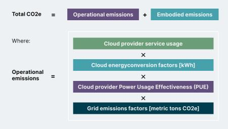
and: Embodied Emissions = estimated metric tons CO2e emissions from the manufacturing of datacenter servers, for compute usage First, the application establishes cloud usage via provider billing data. Second, it estimates energy used by leveraging a similar process to the Cloud Jewels methodology. Finally, the application converts estimated kilowatt hours into estimated CO2e. These processes are inevitably improved and refined on an ongoing basis.
