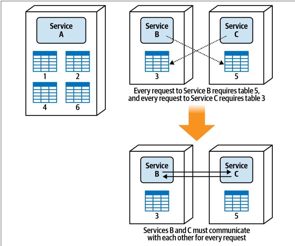
Figure 7-17. Database table relationships impact service granularity
