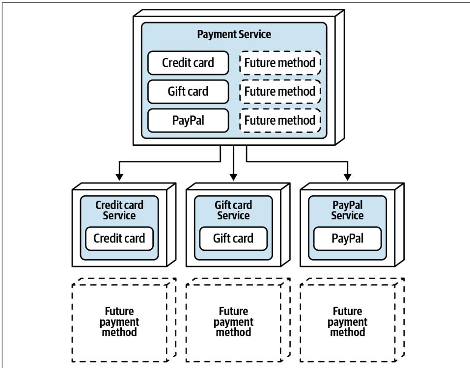
Figure 7-8. Planned extensibility is a good disintegration driver
