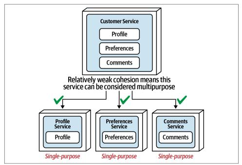
Figure 7-3. A service with relatively weak cohesion is a good candidate for disintegration
