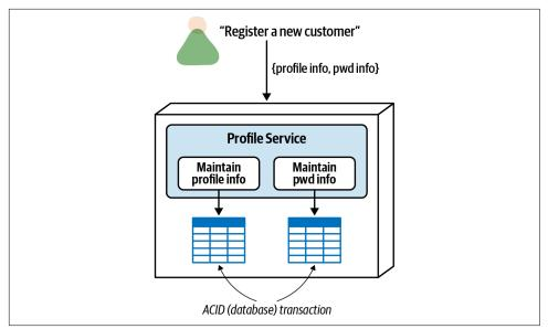
Figure 7-11. A single service supports database (ACID) transactions
