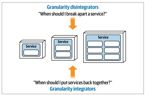
Figure 7-1. Service granularity depends on a balance of disintegrators and integrators
