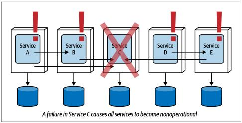
Figure 7-12. Too much workflow impacts fault tolerance
